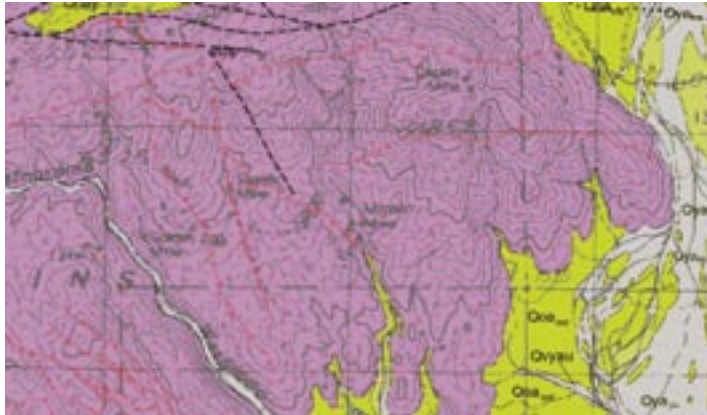
Geology of the mission mine area. purple = jurassic-cretaceous granites, red = veins, yellow = alluvium
